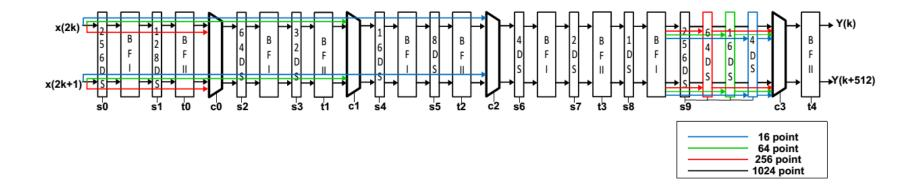
Four different architectures are combined to generate one reconfigurable architecture using only a few additional switches and wires.
