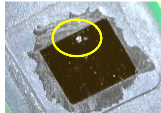
Fig. 4 : Damaged circuit (hole in silicon)
