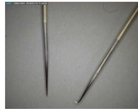
Fig. 5 : New and damaged probe tip ends
